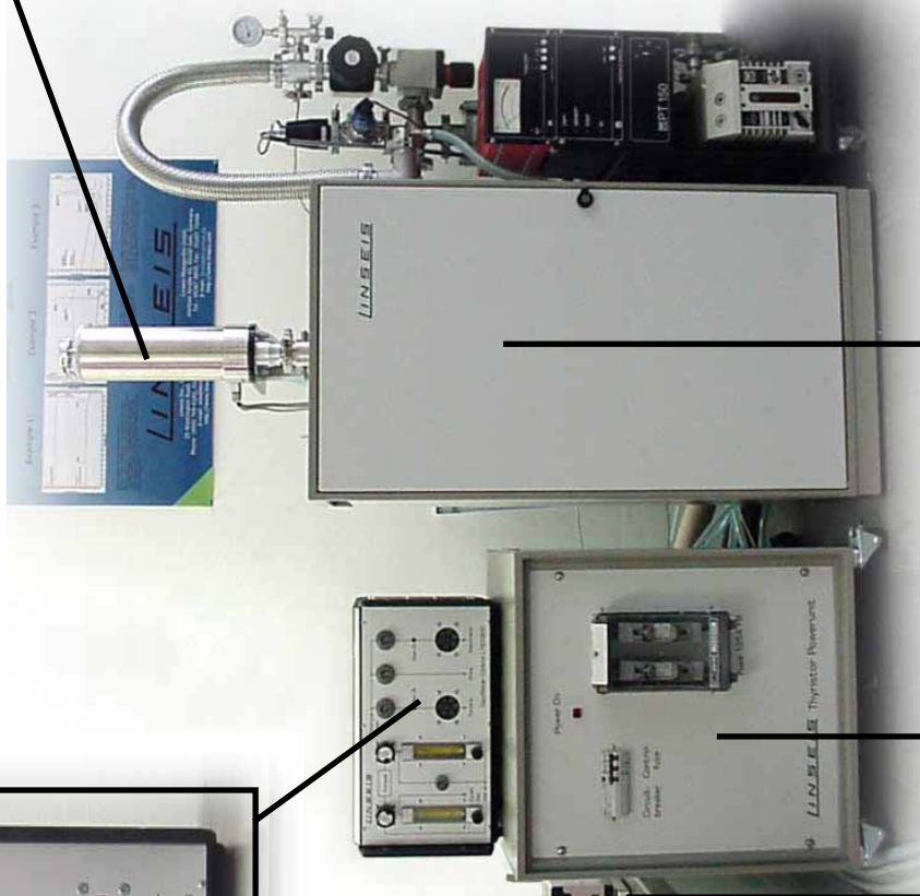
2 times gas control with integrated 3 times water control, for furnace, dilatometer and pump.
