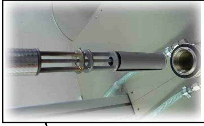
Tantal measuring system for temperature range up to 1800°C.
